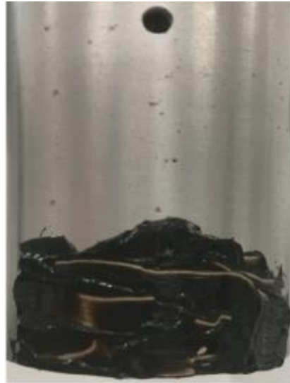
Figure 3. Sleeve covered with tar oil.
